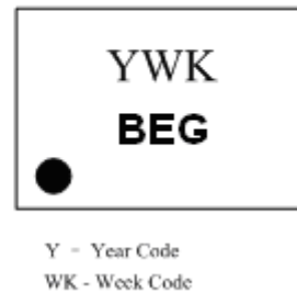
MSOP8/SOP8 Marking (Top View)
