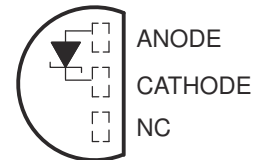
1.2 V ... LP (TO-92/TO-226) PACKAGE (TOP VIEW)
