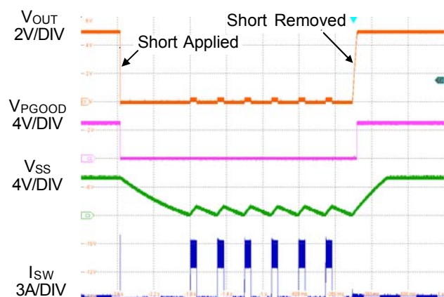
Figure 3. Short Circuit Protection and Recovery
