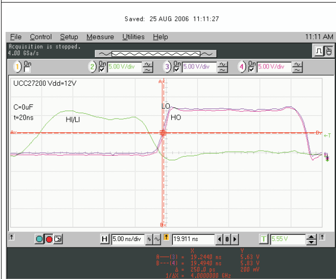
Figure 32. 20-ns Input Pulse Delay Matching
