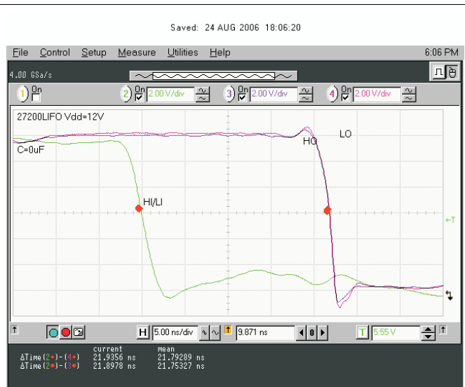
Figure 31. V_{LO} and V_{HO} Falling Edge Delay Matching
