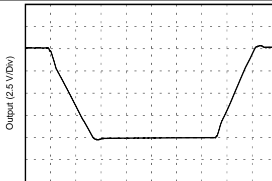
Figure 32. Small-Signal Step Response
