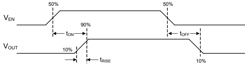
Figure 3. SGM2588A/C/E/G//K Switch Turn-On and Turn-Off Delay Times
