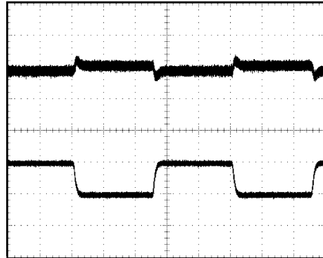
V_{\text{IN}} = 12\text{V} , V_{\text{OUT}} = 3.3\text{V} , I_{\text{OUT}} = 300\text{ mA to } 200\text{ mA to } 300\text{ mA} Top trace: V_{\text{OUT}} , 20 mV/div, AC Coupled Bottom trace: I_{\text{OUT}} , 100 mA/div, DC Coupled T = 200\ \mu\text{s/div}
