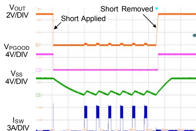
Figure 3. Short Circuit Protection and Recovery
