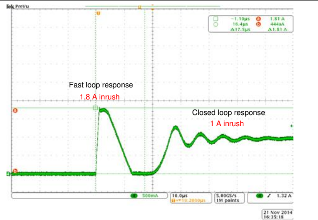
Figure 49. Hard Short-to-GND Waveform
