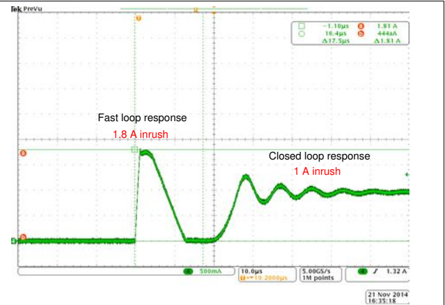
Figure 49. Hard Short-to-GND Waveform
