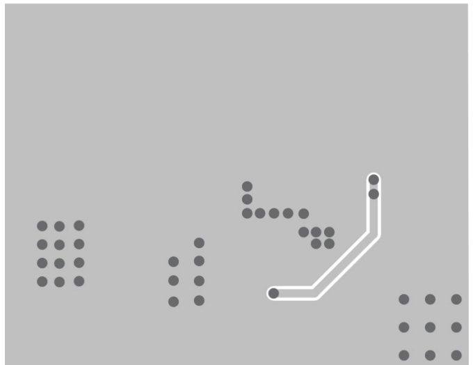
Figure 8. PCB Bottom Layer
