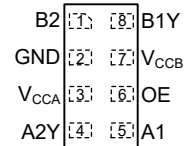
Figure 5-2. DTT Package, 8-Pin SON Transparent (Top View)
